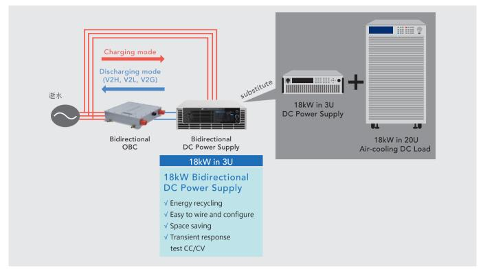
Bidirectional on-board charger testing configuration
