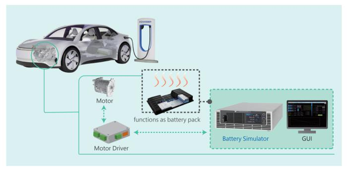
Start-stop system motor driver test application
